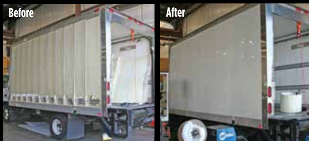
Refrigerated truck body repairs
