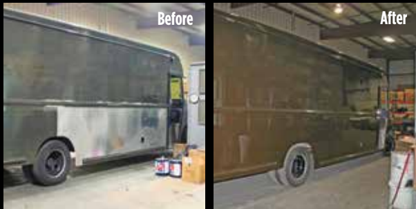
Fabricate and replace body panels
