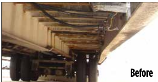
Repair Structural Damage and Corrosion to Frame, Cross-Members and Decks; Reroute Wiring and Hydraulics
