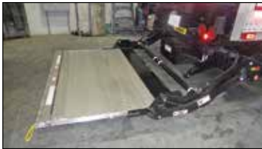
Recent Installation of a New Maxon Slider Lift Gate onto a Semi-Trailer
