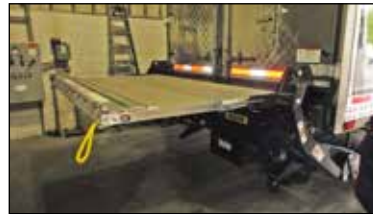
Recent Installation of a New Maxon Slider Lift Gate onto a Semi-Trailer
