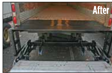
Recent Installation of a New Maxon Slider Lift Gate onto a Semi-Trailer
