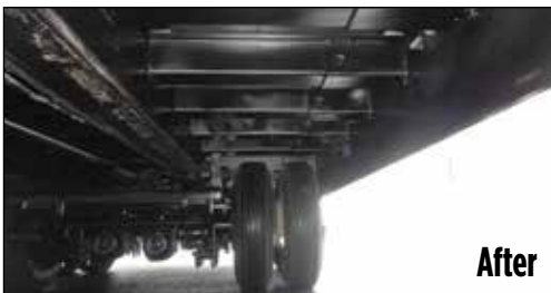
Repair Structural Damage and Corrosion to Frame, Cross-Members and Decks; Reroute Wiring and Hydraulics
